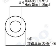
适用螺纹或孔径 Thread or Thru Hole Code : 2-56, 4-40, 6-32, 8-32, 116, 143, M2, M2.5, M3, M3.5, M4, 3.6, 4.2
