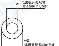
适用螺纹或孔径 Thread or Thru Hole Code : 2-56, 4-40, 6-32, 8-32, 116, 143, M2, M2.5, M3, M3.5, M4, 3.6, 4.2
